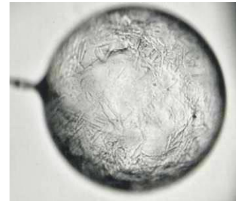
T_A = 14,5 K Solid phase (focus on the front surface of the capsule)
