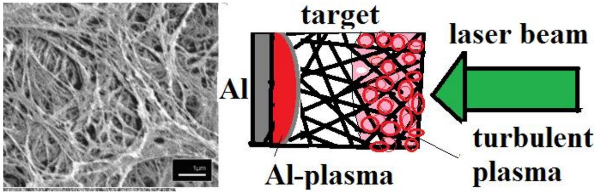
Fig.1. Left side: image of cellulose triacetate (TAC) matter with  $\rho \sim 10 \text{ mg/cm}^3$ , right side: scheme of laser beam–foam interaction, formation of hot turbulent plasma formation. A foam matter placed on thin aluminum base.
