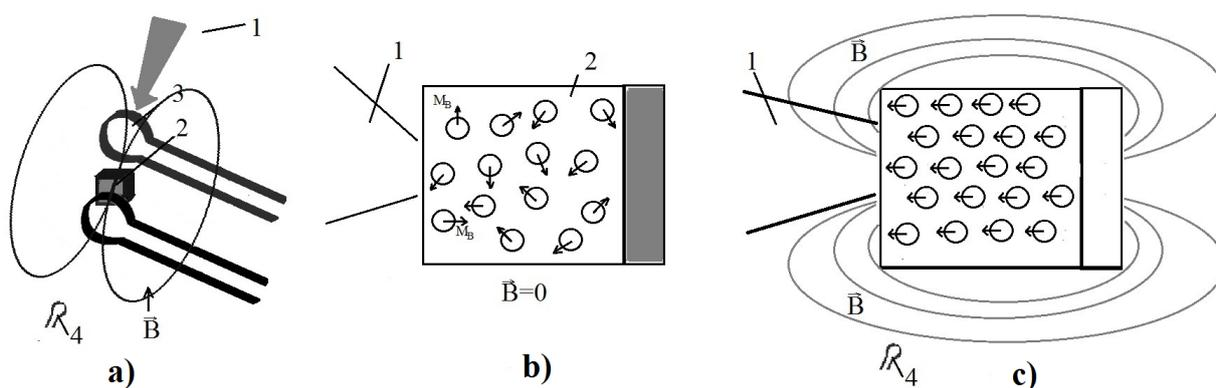
Fig.2. A scheme of external magnetic field production near laser target (a), porous target on mount and magnetic moments ( $M_B$ ) distribution in turbulent laser plasma without external field (b), magnetic moment reorientation under action of external magnetic field into turbulent plasma (c). 1 – laser beam, 2 – target 3- installation, which has produced the external field, 4 – diagnostic probe,  $B$  – magnetic strength lines of magnetic field.
