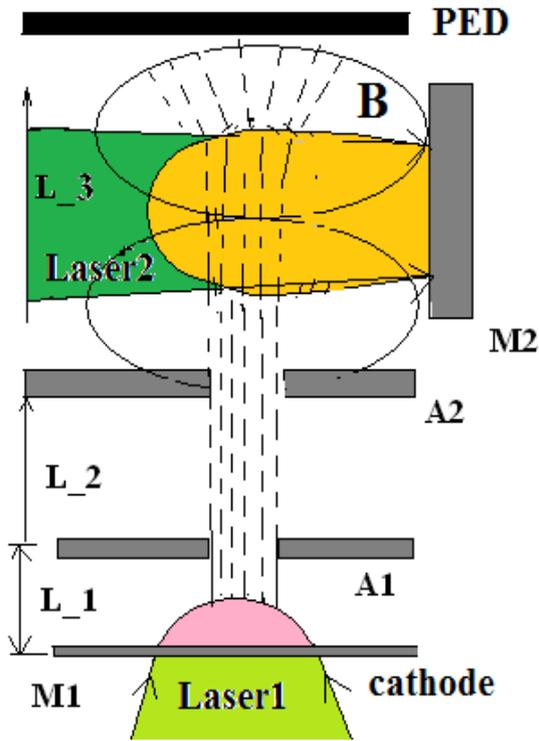
Fig.3. A design of diagnostic e-bunch formation. Laser1 – laser beam, which has formed hot plasma for e-bunch formation, M1 – target for hot plasma formation, A1, A2 – the first and the second anodes. Laser2 – laser beam, which has formed turbulent plasma. M2 – porous target, which has formed turbulent plasma with internal magnetic fields, PED-Photo-electronic device, L\_1, L\_2, L3 – interspaces between electrodes
