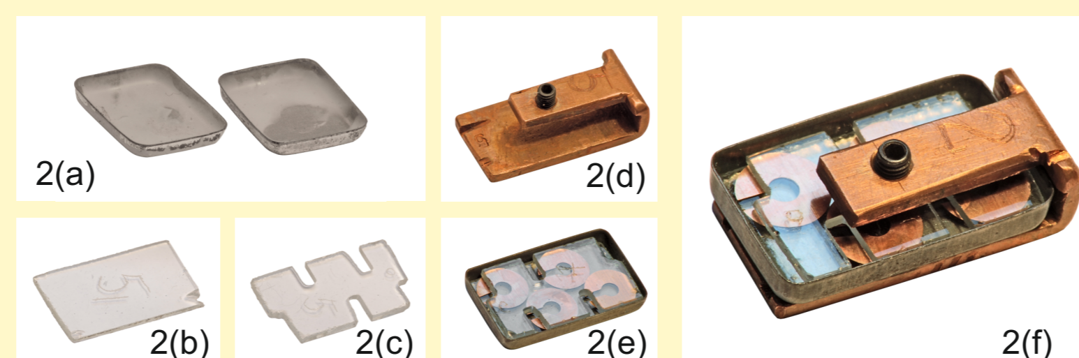
Scheme 2 Assembly device for drying between the plates 2(a) a pallet 2(b) a glass slide 2(c) the cover glass with recesses for drying between the plates 2(d) a clamp 2(e) stacking targets 2(f) general view of the Assembly
