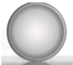
Cryogenic target with the ultra-fine D_2 layer
