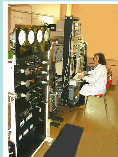
Fill facility: Filling of CH shells with gaseous fuel up to 1000 atm at 300K
