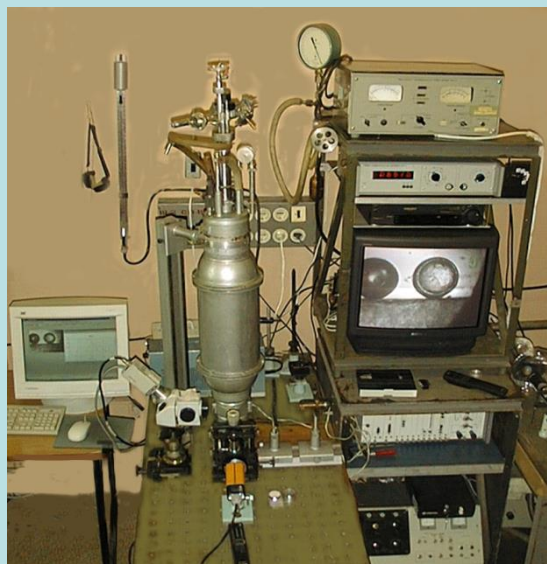
Layering module (LM): FST method for fuel layering inside free-rolling targets
