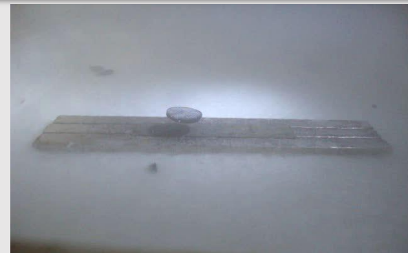
\text{YBa}_2\text{Cu}_3\text{O} pellet of 12.4 mm-diam, 1-mm-thick
