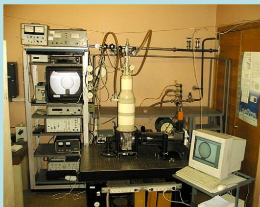
Cryogenic target characterization: 100-projections visual-light tomograph with 1 um space-resolution
