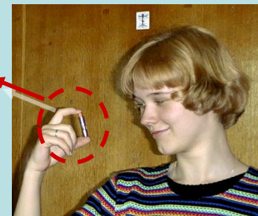
Handheld Shell Container (SC) for fuel filled shells transport at 300 K from the fill system to the FST-layering module
