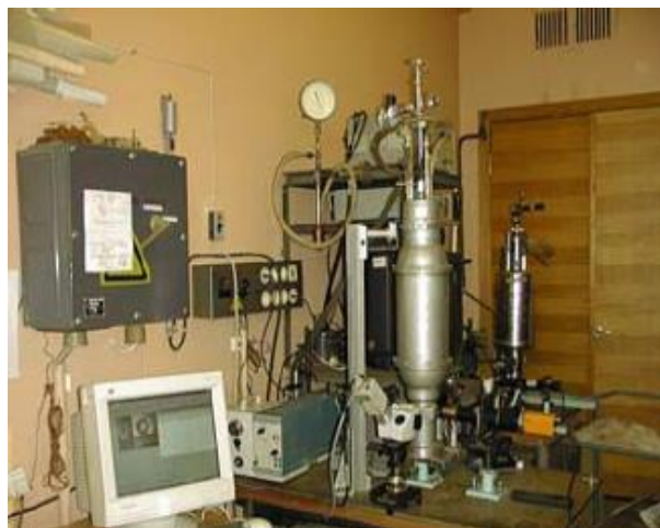
■ FST layering module for fabrication of isotropic ultra-fine fuel layers inside moving free-standing targets
