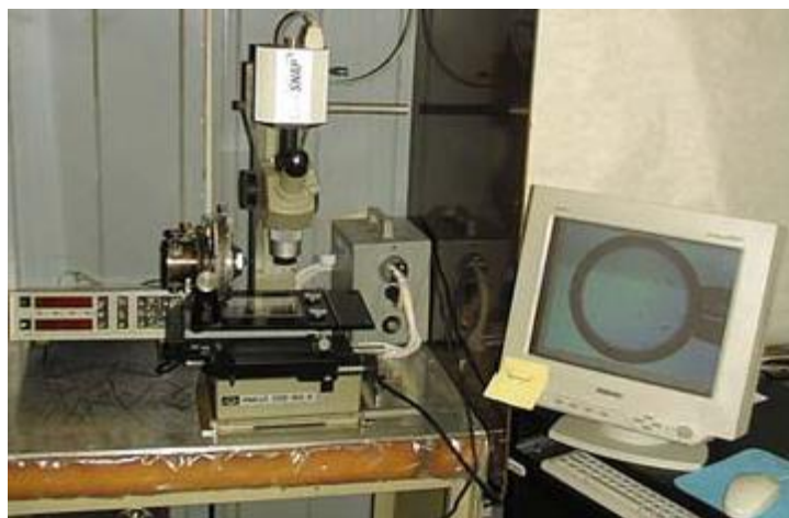
■ Video and tomography shell control before the shell filling with a gaseous fuel
