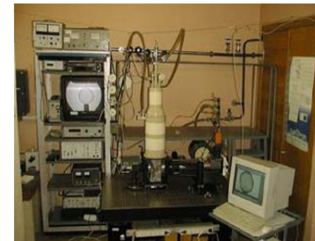
■ Video and tomography control of the cryogenic targets (100 projections, 1- \mu m spatial resolution)
