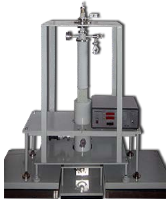
Cryogen-free cryostat for optical, X-ray and Mossbauer studies
