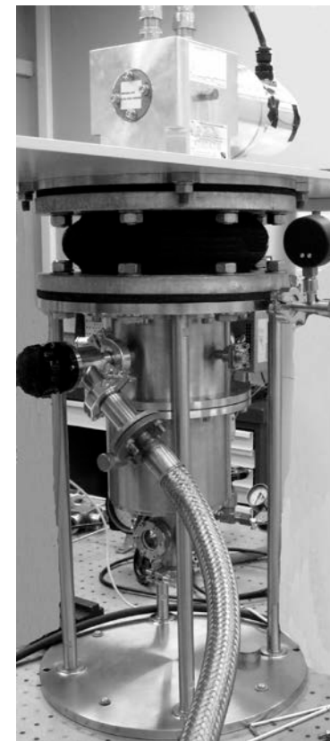
Fig.3. The optical cryostat developed by our group ( < 1 \mu\text{m} vibrations)
