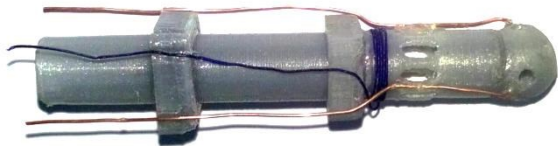
Model of cryogenic target printed using additive technology
