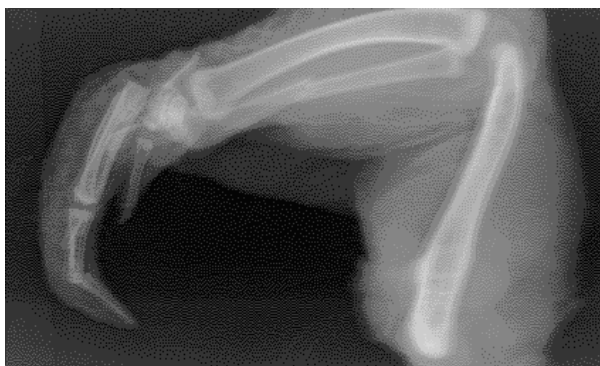
Fig.1. X-ray picture of a chicken wing obtained with the help of a cathode based on CNTs from kovar
