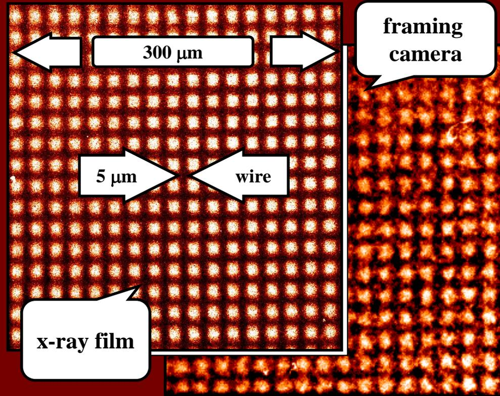
The resolution of the x-ray optical system reaches 2  $\mu\text{m}$
