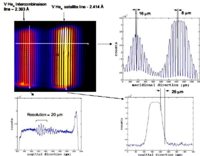
FIG. 2: Monochromatic image of a 400pi gold grid in the backlighting scheme see figure 1.b. The densitograms of the image in the sagittal and meridional direction at  $2.393\text{\AA}$  and at  $2.414\text{\AA}$  are also presented. The hole in the grid refer to the target chamber center.
