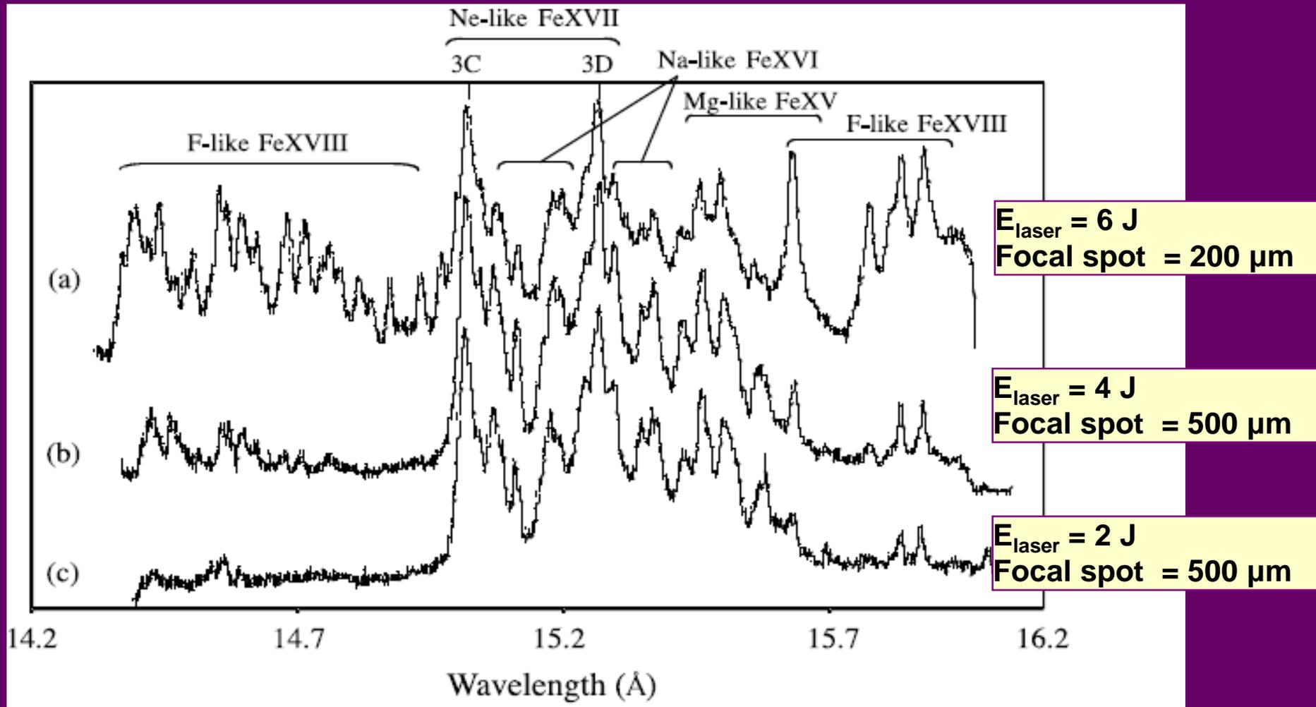
Typical X-ray spectra of Fe between 14 and 16 Å obtained in plasmas produced by the 15 ns Nd:glass laser (Tor Vergata University, Rome, Italy)
