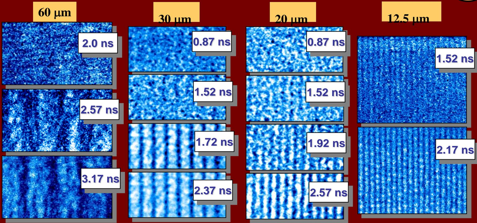
The use soft 1.47 keV x-rays used allows small amplitude perturbations to be observed.
