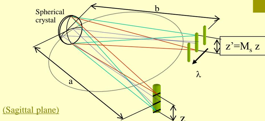
Two dimensional spatial resolution gives a very important information about radiation properties of different ions inside the plasma expansion plume (the angle distribution of ions acceleration could be measured)
