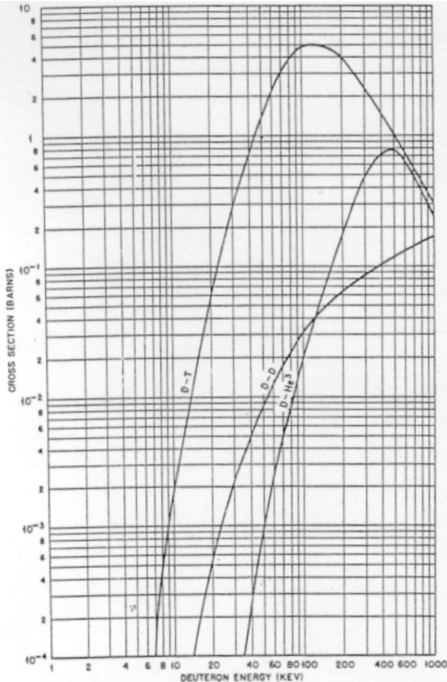
Cross sections for D-T, D-D (total), and D-He<sup>3</sup> reactions.
