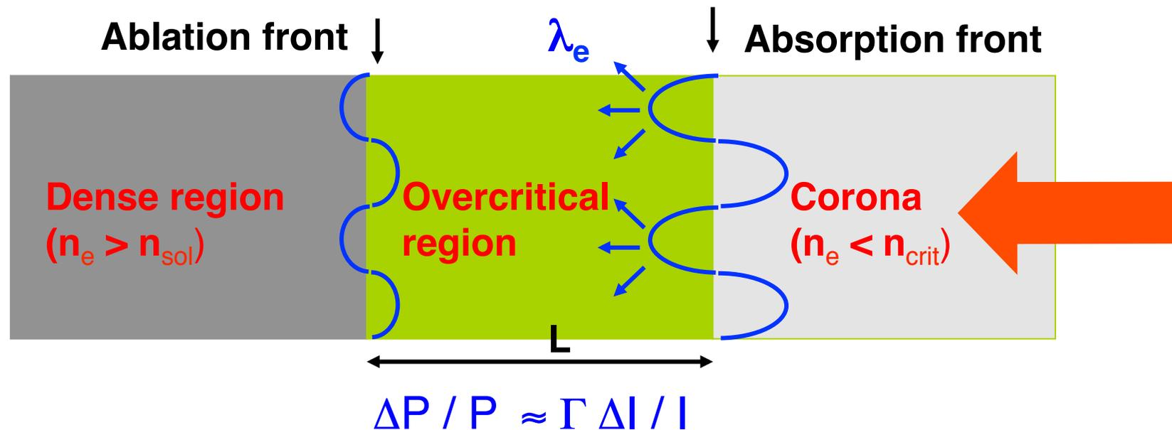
Non-uniformities present at the laser absorption surface are reduced at the ablation surface by
