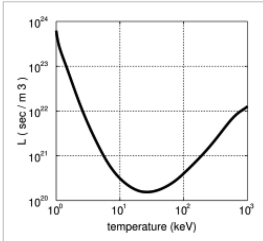
Is function of T and has a minimum at  $\approx 25$  keV ( $2.9 \cdot 10^8$  K) for  $D + T \rightarrow {}^4\text{He} + n$
