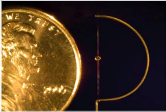
*Figure 3.3:* The laser-fusion targets used on OMEGA experiments are typically ~1 mm in diameter and are suspended by spider silks.
