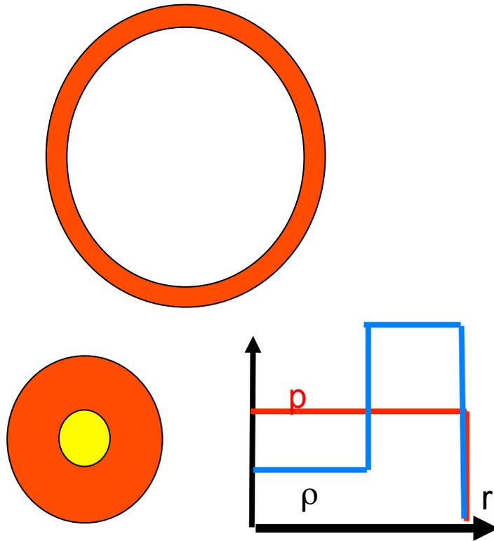
Stagnation is reached as the pressure of the internal fuel increases and gradually slows the shell down.
