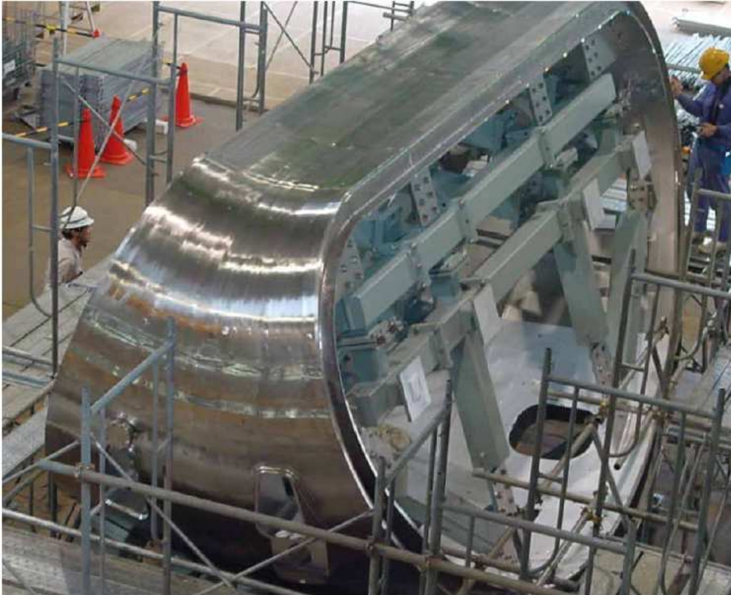
The first 40° sector of the JT-60SA vacuum vessel was completed in June 2011 at JAEA Naka Fusion Institute, JAPAN
