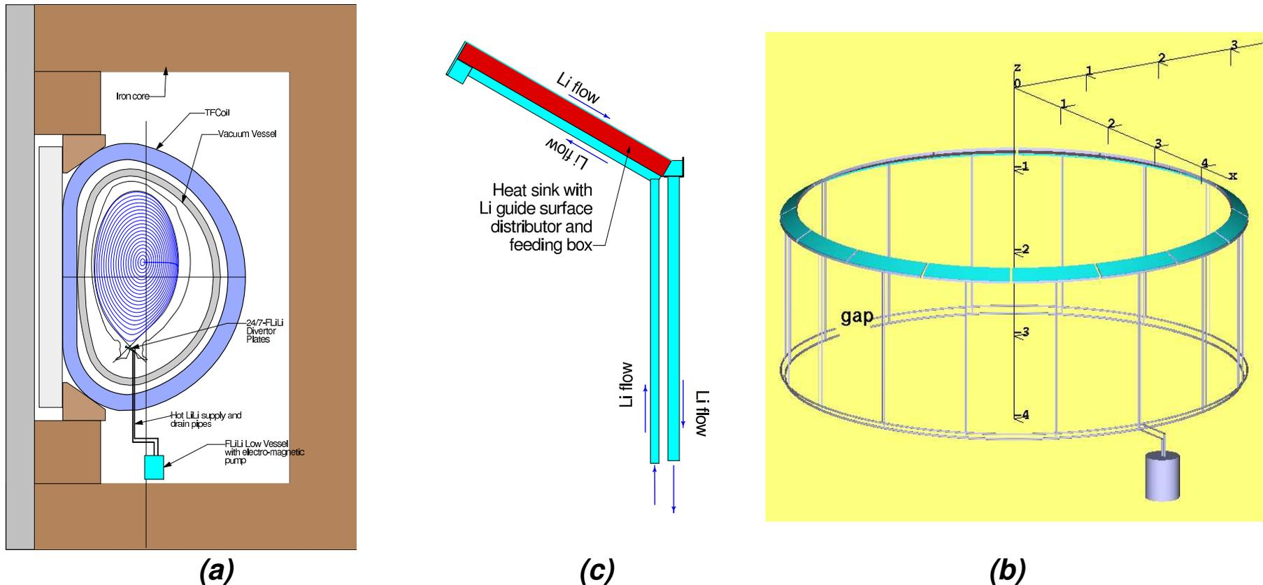
**Figure 2. (a) Relative position of the 24/7-FLiLi target plate inside the JET vessel and “lithium plumbing” inside the iron core. (b) 3-D view on entire 24/7-FLiLi system with a single lower vessel, controlling the flow, and horizontal drain/supply ring pipes.**
