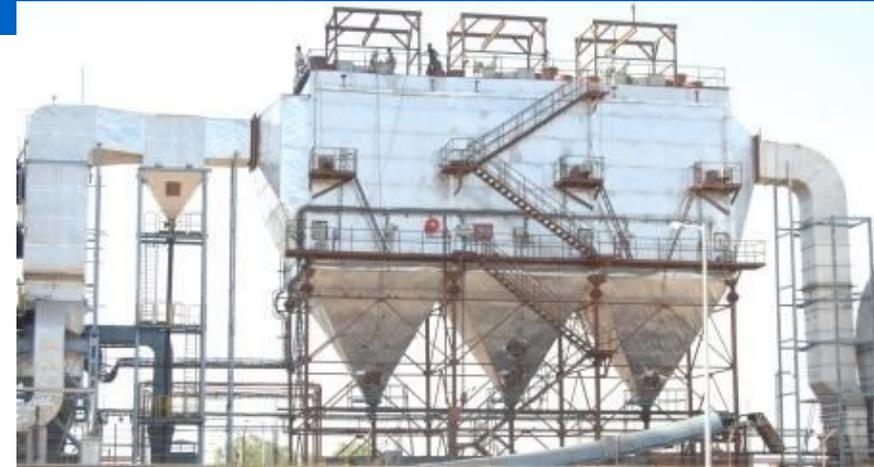
Dust particles become charged in plasma, are attracted to electrodes, and come to the collector (analogue of “divertor” in tokamacs)
