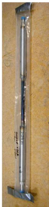
Sample assembly ( $\text{Er}_2\text{O}_3$ -coated)
